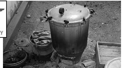
The pressure cooker they use to sterilize surgical instruments. It is done outside on a make shift kerosene stove.
